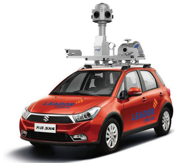
Figure 6. The mobile mapping vehicle system developed by Leader Spatial Information Technology Corporation.
