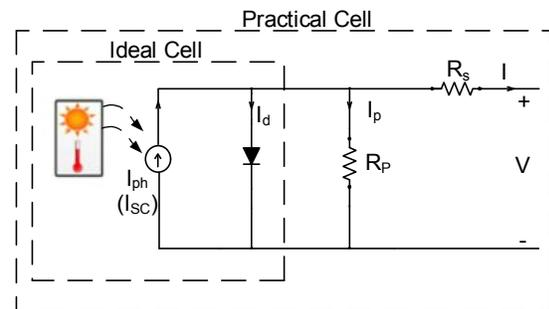
Fig. 2. Equivalent circuit of photovoltaic cell
