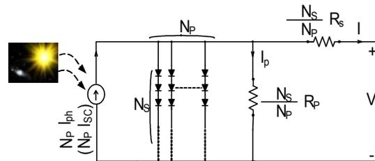
Fig. 3. Equivalent circuit model of solar PV array
