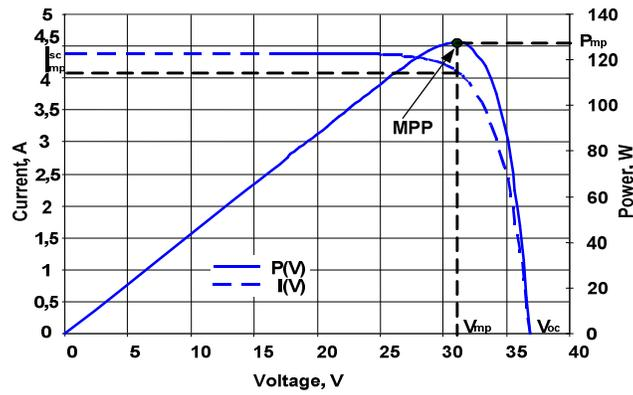
Fig 5. Characteristics curve of a typical PV cell
