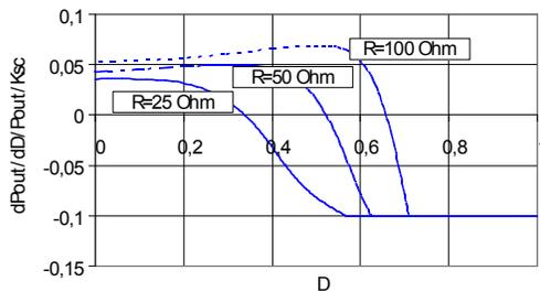
Fig. 10. Modified function for calculation of  $\Delta D_i$  for single system
