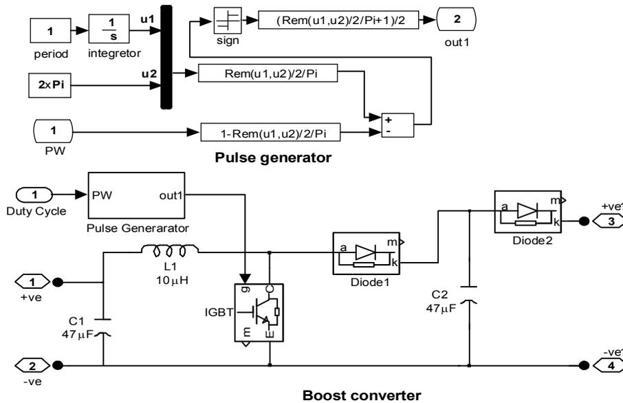
Fig. 7. Simulink-model of Boost DC-DC converter
