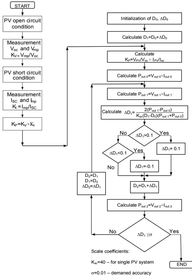
Fig. 6. Flowchart of hybrid MPPT algorithm
