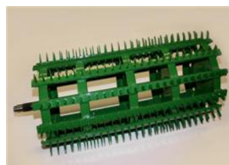
Fig. 1. Spike tooth type threshing cylinder
