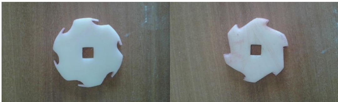
Fig. 4. Shapes of cells in metering unit (a) Shape 1- extended oblong ;(b) Shape 2- oblong
