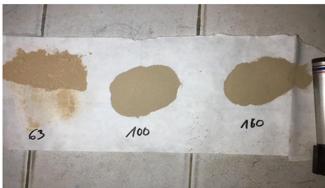
Fig. 1. Photograph of merchant phosphate in grain sizes 63; 100; 160 μm
