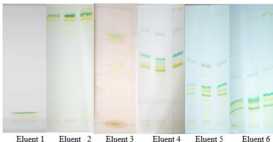
Fig. 3. Eluent of optimization for Thin layer Chromatography
