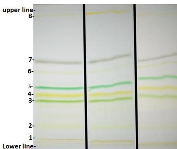
Fig. 6. TLC chromatograph of crude extract from tomato crop leaves at different growth stages
