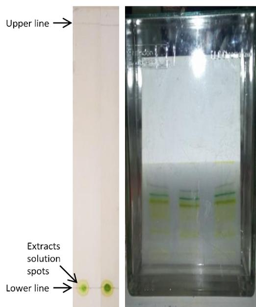
Fig. 2. TLC test set up
