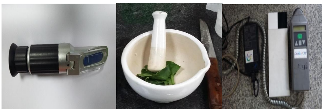
Fig. 2. Hand refractometer, pestle and mortar to measure TSS of vegetables and hunter colorimeter-colour Tec-PCM™ colorimeter
