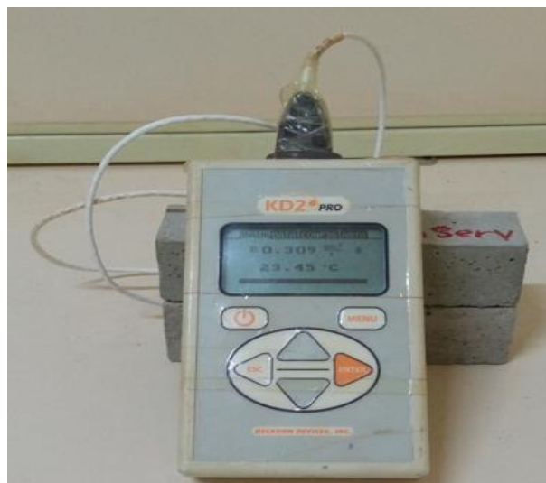
Fig. 3. Measurement of thermal properties with KD2-Pro
