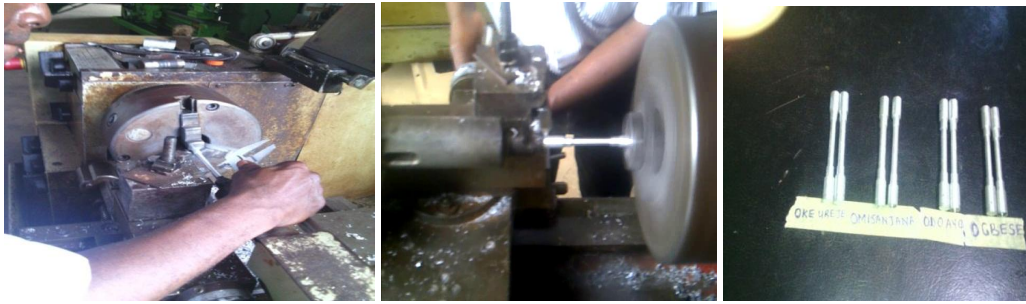
Fig. 4. Production of Tensile Specimens on Lathe Machine
