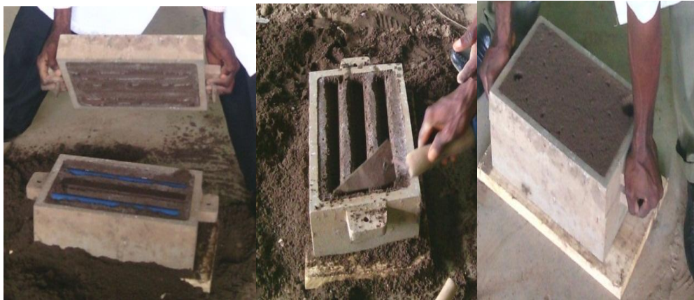
(g) Opening of mould to remove the patterns (h) Dressing & gating the mould. (i) Covering of the mould & ready for casting.
