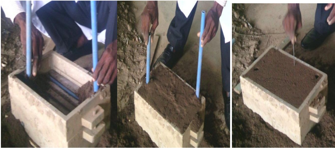
(d) Placing of cope over drag (e) Removing of runners & riser (f) Venting of the mould
