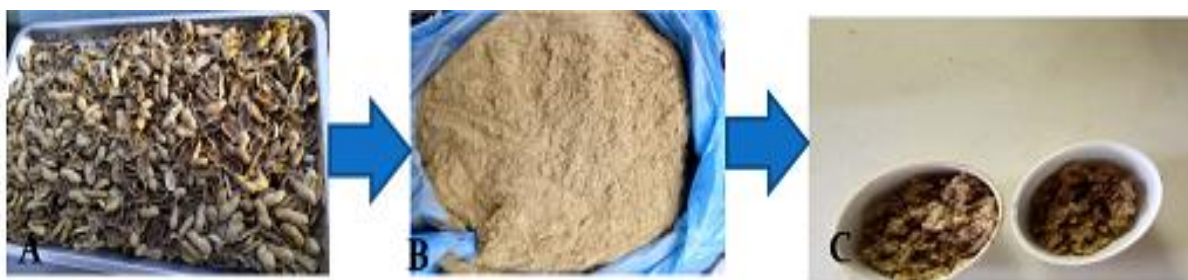
Fig. 1. A. Groundnut shells B: Pulverized groundnut shells C: Groundnut Shell Coagulant (GSC)
