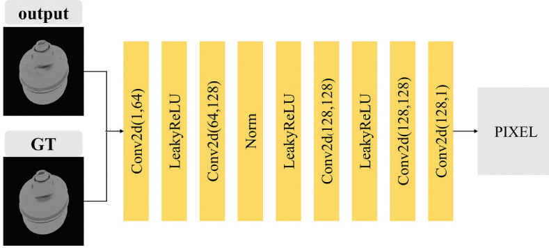
Figure 7. The structure of the pixel discriminator. Conv2D (a, b) means the input channel of the convolution layer is a, and the output channel is b.
