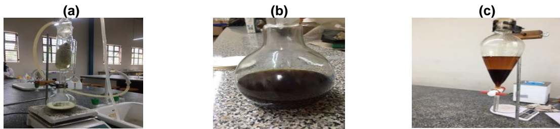
Fig. 3. Shows various stages of biotransformation (a) Soxhlet extraction of oil from pumpkin (b) Crude trans-esterified mix of pumpkin seed oil and (c) Separated crude trans-esterified seed oil
