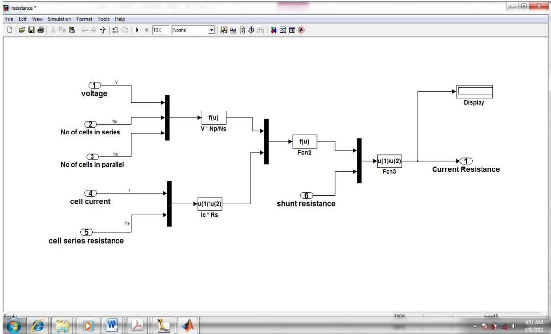
Fig. 2.8. Subsystem of the generated voltage current model
