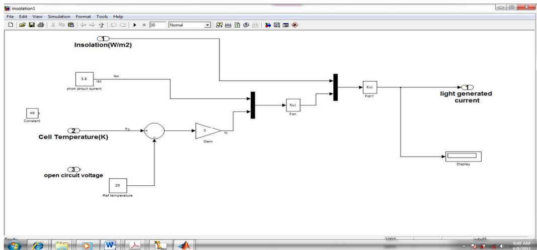
Fig. 2.7. Subsystem of the generated panel current model
