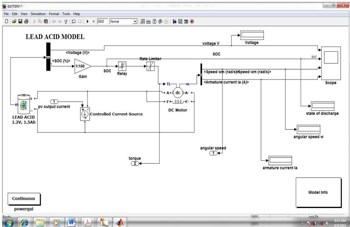
**Fig. 2.11. Subsystem of the solar car battery model**
