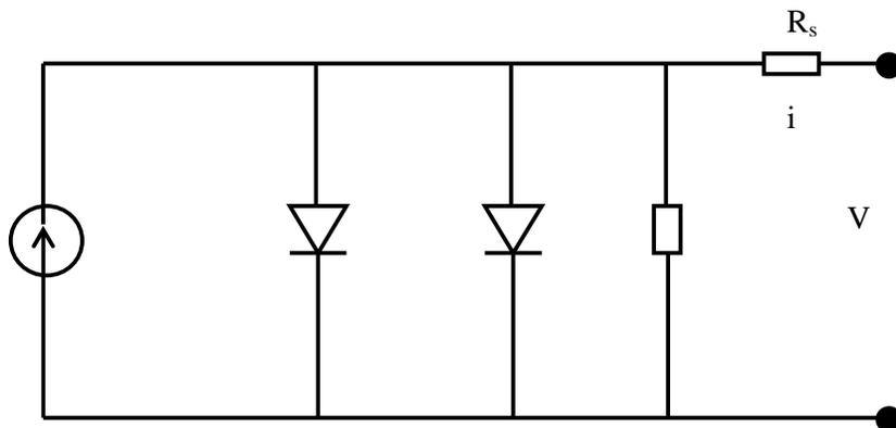
Fig. 2.2. Equivalent circuit for a double exponential model for a PV Panel
