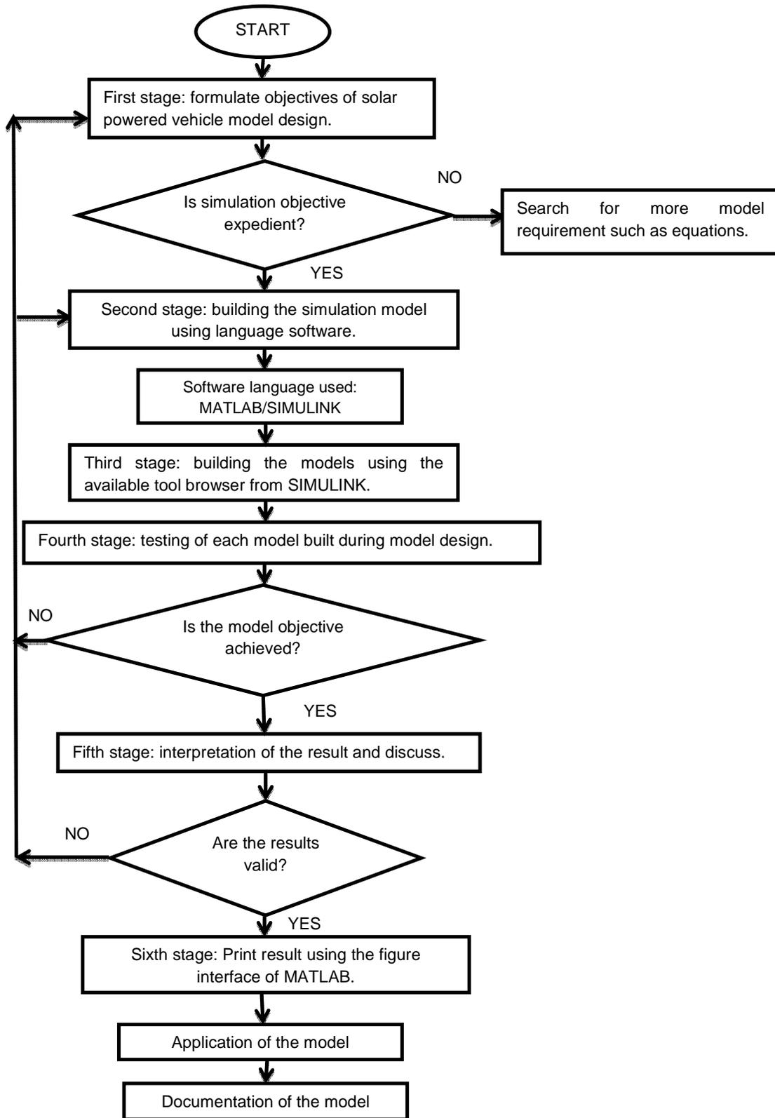
Fig. 2.6. Solar powered vehicle simulation model flowchart
