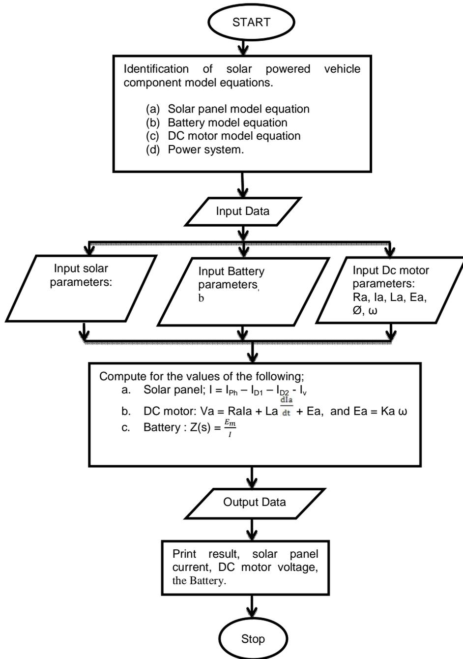
Fig. 2.4. Flow chart showing the relationship of the mathematical model of SPC
