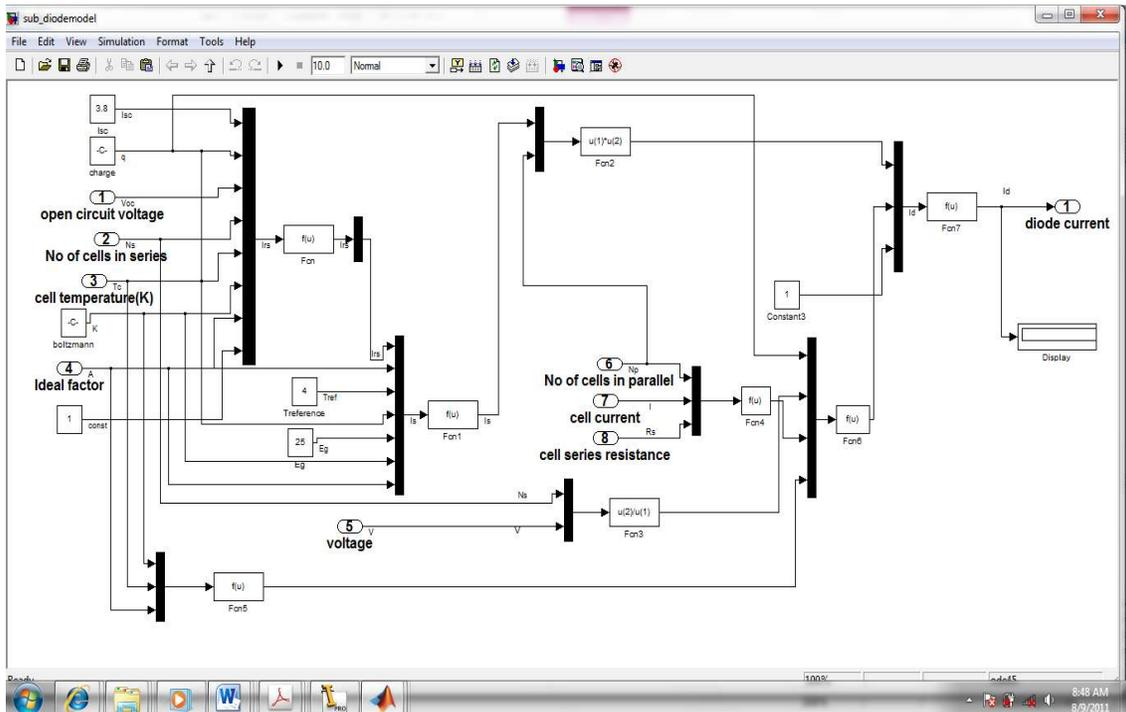
Fig. 2.9. Subsystem of the diode current model
