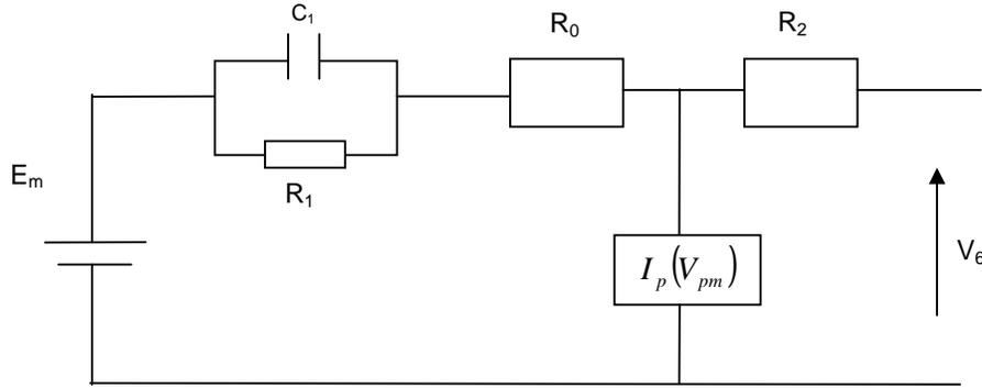
**Fig. 2.3. Equivalent circuit for a lead and battery**
