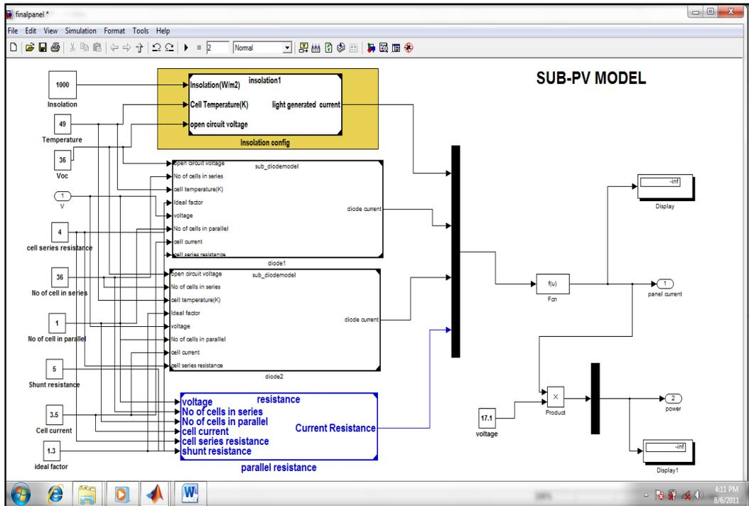
Fig. 3.1. Simulink implementation of the expression of PV panel
