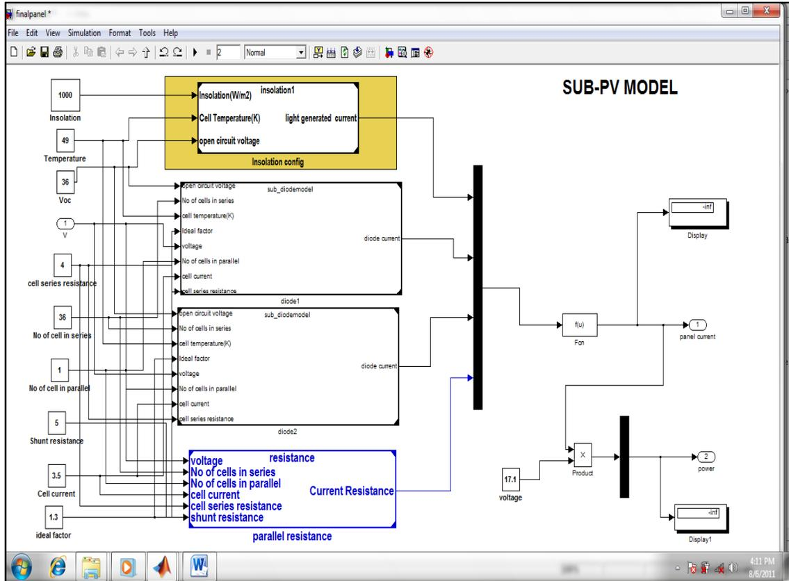
Fig. 2.6. Subsystem of the solar panel model
