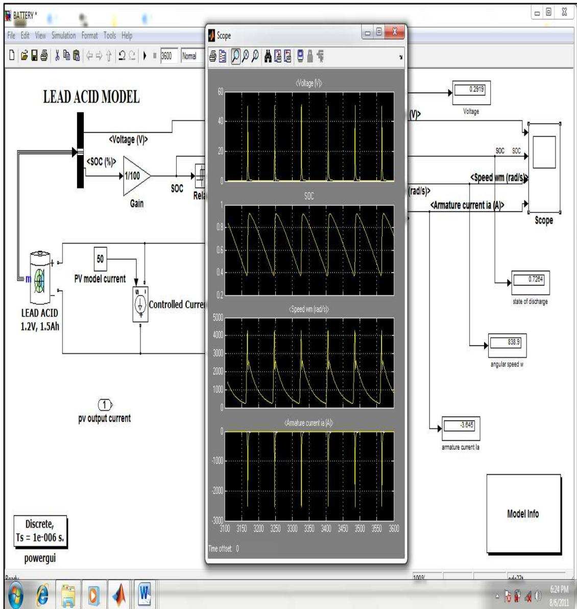
Fig. 3.3. Simulink implementation of the expression of battery and Dc motor
