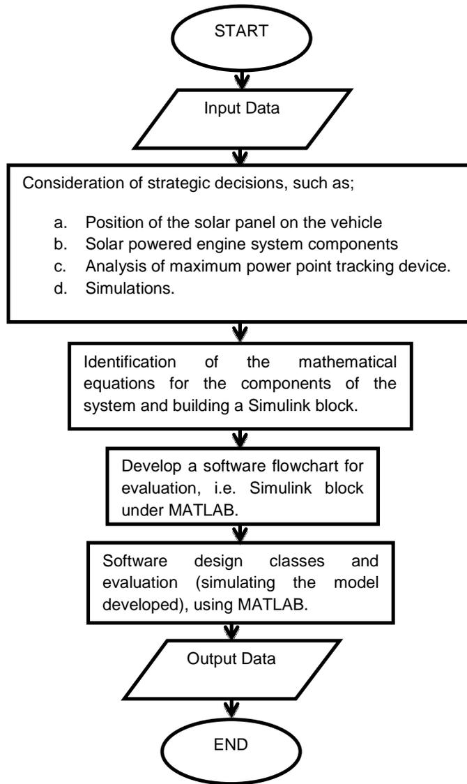
Fig. 2.1. Solar powered engine simulation model design procedure
