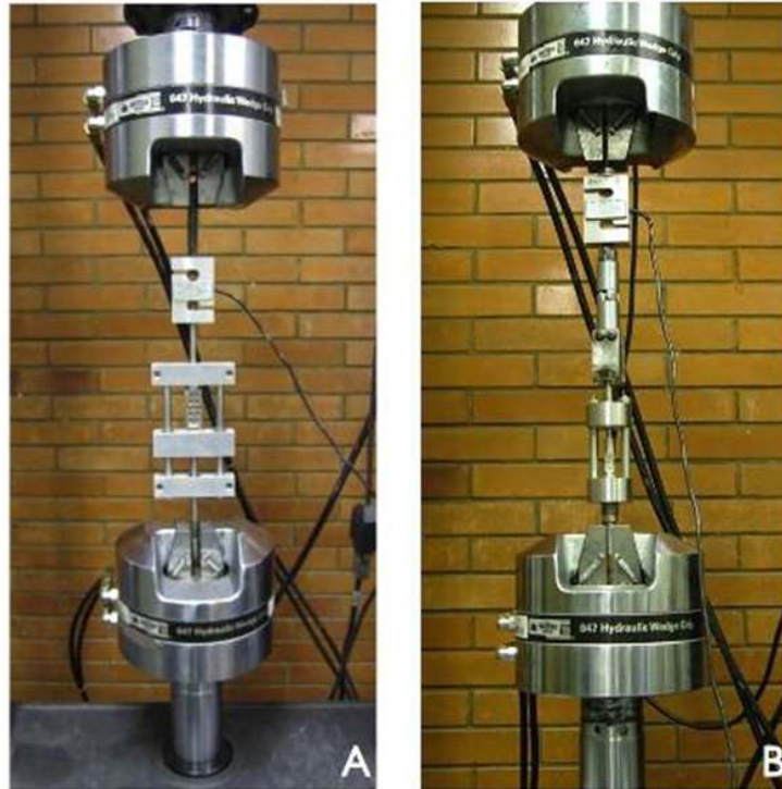
Fig. 4. (A) The Flextest device mounted on the MTS universal testing machine with a load cell with a nominal capacity of 100 kg. (B) the Bencor Multi-T device mounted on the MTS universal testing machine with the same load cell
