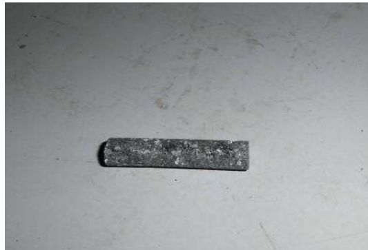
Fig. 5. Pitting corrosion of sample in acidic medium
