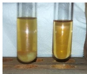
Fig. 31. Phenols test- Yellow color precipitate present at the bottom of the test tube
