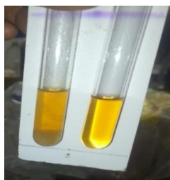
Fig. 29. Alkaloid test- Brown precipitate present at the bottom of the test tube
