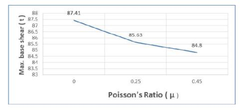
Fig. 13. Relation between poissons ratio value and the max. base shear (20 – Story building)
