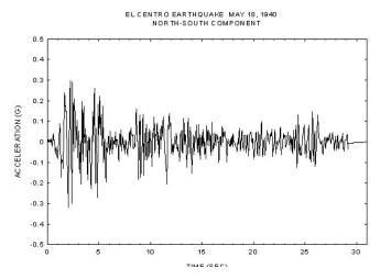
Fig. 1. A plot for the time history of the ground acceleration, velocity and displacement of El-Centro records
