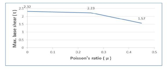
Fig. 9. Relation between poissons ratio value and the max. base shear (10 – story building)
