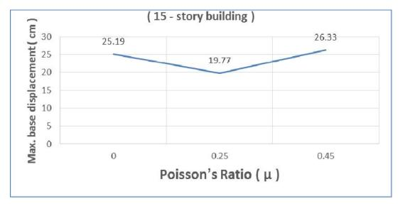
Fig. 10. Relation between poissons ratio value and the max. base displacement (15 – Story building)
