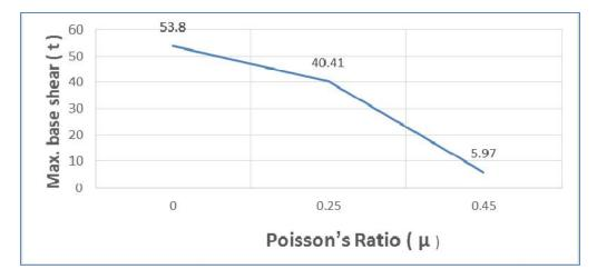
Fig. 11. Relation between poissons ratio value and the max. base shear (15 – story building)
