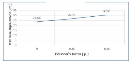
Fig. 8. Relation between poissons ratio value and the max. base displacement  $(10 - story \ building)$
