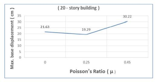
Fig. 12. Relation between poissons ratio value and the max. base displacement
