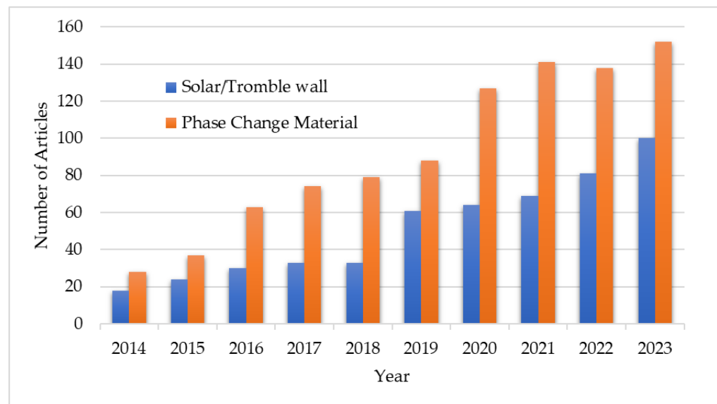
Figure 1. Trends in published articles by year on Trombe walls and phase-change materials from 2014 to 2023 [53,54].
