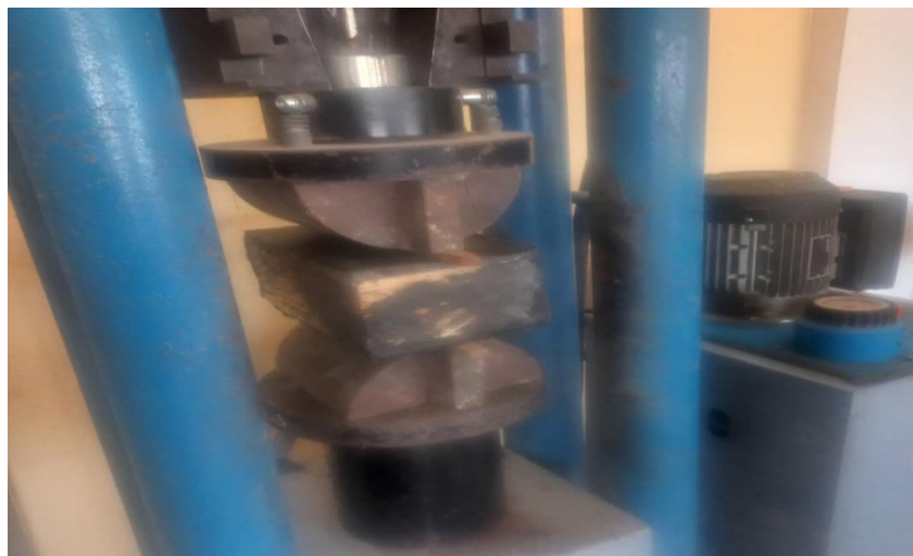
Fig. 4. Split tensile test of plastic brick
