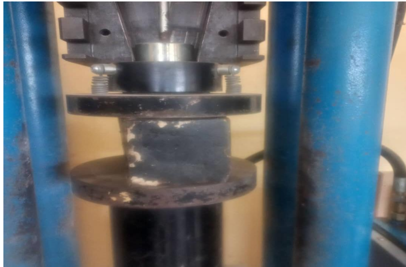
Fig. 3. Compressive strength test of plastic brick
