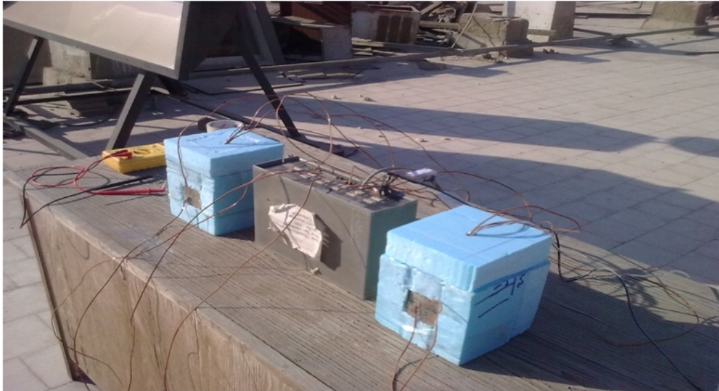
Fig. 4. Test set up for both K and U values
