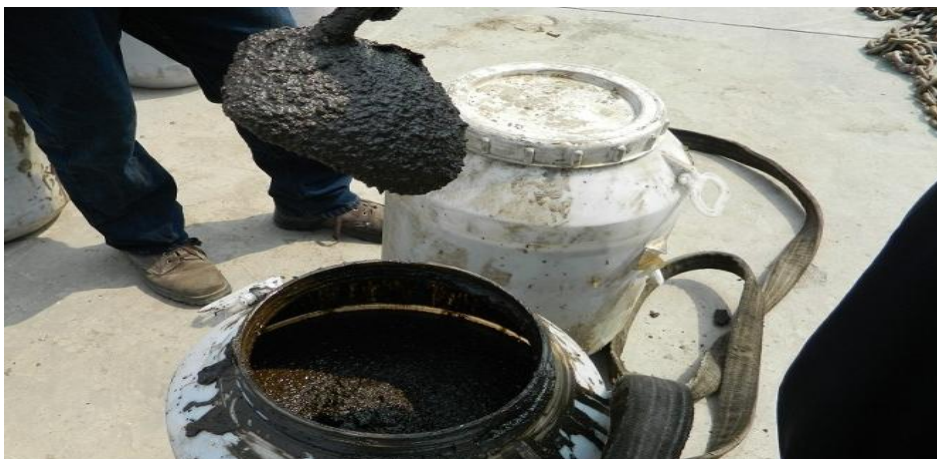
Fig. 3. J.1. Sample of drill cuttings before treatment
